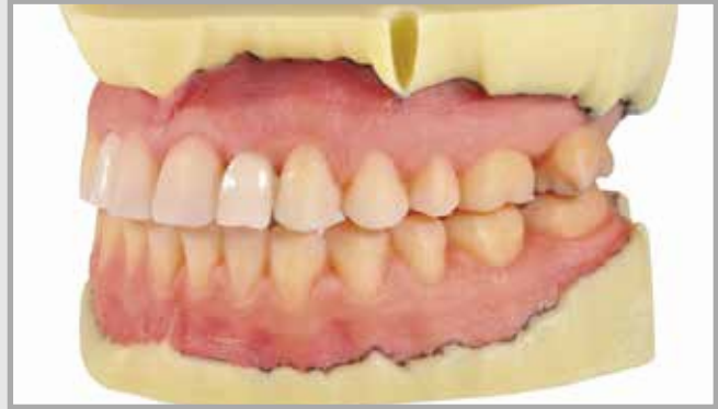
Fig. 2: PolyJet technology (J750 Digital Anatomy Printer; Stratasys) allows complex printing of multi-color and multi-texture structures in a single-print operation.
