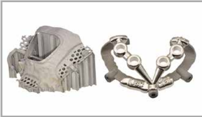
Fig. 3: Selective Laser Melting (SLM) allows direct metal printing of cobalt-chrome (Co-Cr) removable partial dental prosthesis framework and surgical template (part of the surgical template shown was milled).
